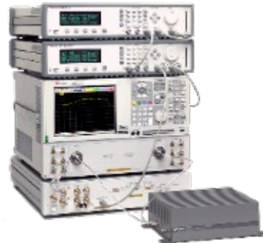
Figure 2. The PNA Series replaced the pulsed 8510 with a bench-top solution.
