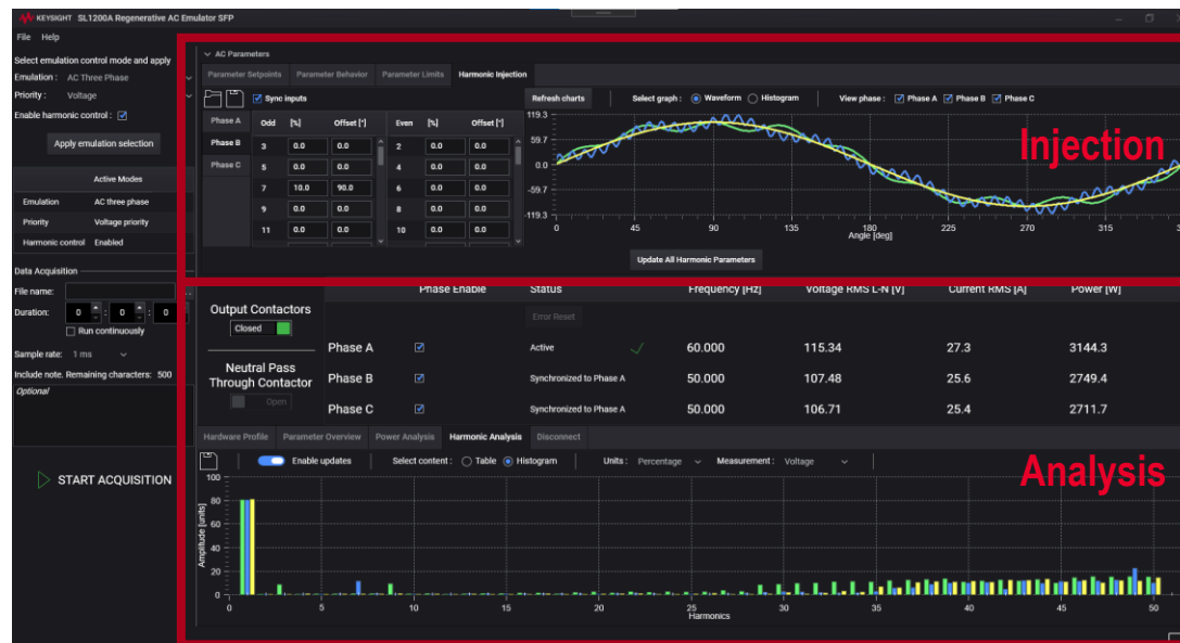
Figure 3. SL1200A Software Front Panel – Harmonics injection and analysis tab
