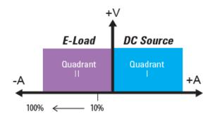
Voltage response APS sourcing current APS sinking current
