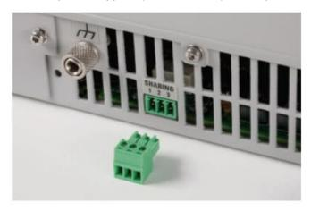
Figure 6. An APS supply's three-wire connection for paralleling multiple supplies
