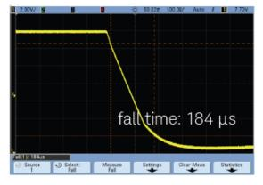
Figure 4. Voltage interrupt pulse generated by N7951A
