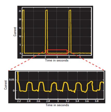
Figure 1. Dynamic current measurement
