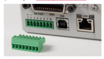
Figure 10. Digital control port on rear panel
