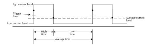
**NOTE** The pulsed waveform in Figure 5 shows trigger level and the high, low, and average times set by the Model 2306 using the auto-time feature.
