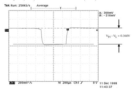
**NOTE** Figure 15 shows the voltage drop during the transmit portion of the pulse of a GSM phone using the Model 2306 battery channel with output impedance set to  $0.24\Omega$ . See Figure 14 for actual Li ion battery results.
