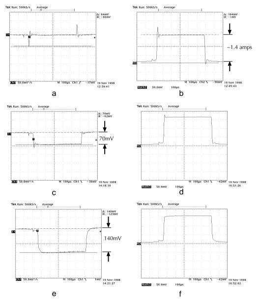
**NOTE** Figure 13 contains the effect of the variable output impedance control of the Model 2306 on the current and voltage performance of a GSM handset.
