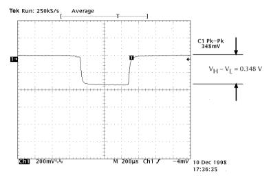
**NOTE** Figure 14 shows the voltage drop during the transmit portion of the pulse with the supplied Li ion battery pack. See Figure 15 for the comparative illustration using the Model 2306.
