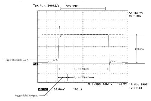
**NOTE** In Figure 6, a trigger delay of 100µs is used to eliminate the effect of a current transient on the pulse current measurement.
