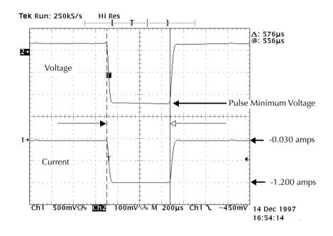
**NOTE** The simulated GSM phone current profile contained in Figure 11 shows a standby current of 0.030A, a transmit current of 1.2A, and the pulse minimum voltage during the transmit frame.
