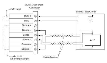
*NOTE* DO NOT jumper the sense inputs and supply outputs at the rear of the supply. DO NOT pass the source and sense leads together in the same twisted pair.
