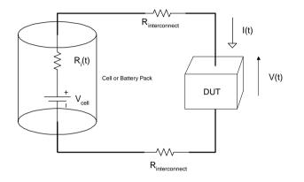
If  $R_{interconnect}$  is small compared to  $R_i(t)$  and if  $R_i(t)$  is relatively constant during the length of the pulse,  $R_i(t) \sim R_i$ , then the voltage across the DUT may be expressed as:
