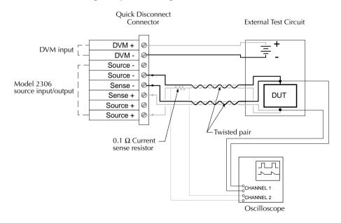
**NOTE** Figure 7 contains a simple circuit for determining the dynamic voltage and current characteristics of the DUT using a 2-channel oscilloscope, a 0.1 ohm resistor used as a current sense resistor, and a voltage probe at the DUT.
